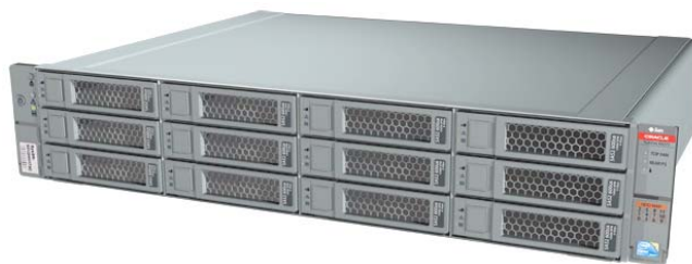
Figure 4: Exadata Storage Server (Exadata Cell)
